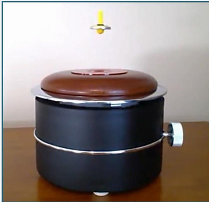
Spin-stabilized magnetic levitation device ( prototype ) Patent No. 9,795,894
